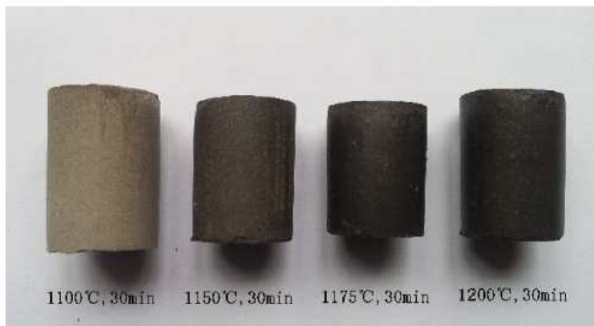
Fig. 5. Photograph of sintered ceramic tiles at various temperatures (pigment sintered with 50% dust+50% \text{Cr}_2\text{O}_3 ).
